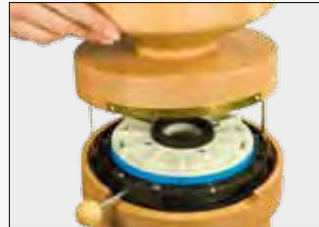
Figure 2 Lift off the funnel.
